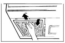
Then pull filter downward and to the front. The filter will drop out.
